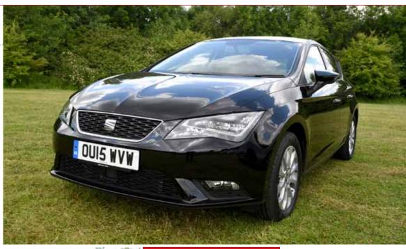
ABOVE: 16-inch alloy wheels and front fog lights with cornering function are standard on Leon SE
