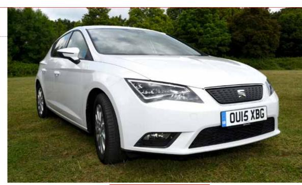
ABOVE: Ecomotive trim includes an aerodynamic front grille to maximise efficiency
