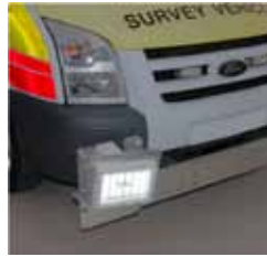
Prototype MarkingCollector device mounted on a survey vehicle
