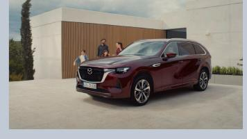
combines a 2.5-litre petrol engine with an electric motor. It delivers a combined output of 327PS and 500nm to all four wheels via an eight-speed automatic transmission.
