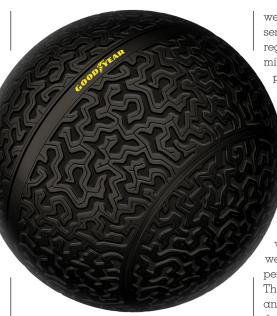
Goodyear Eagle-360 concept tyre relies on magnetic levitation. The tyre is suspended from the car by magnetic fields, similar to magnetic levitation trains, which increases passenger comfort and reduces noise.
