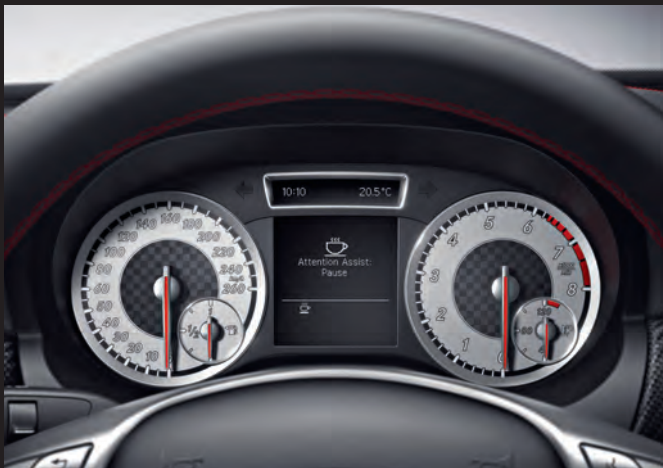
If Attention Assist calculates that the driver is flagging, it sounds a warning alarm and flashes up the symbol of a coffee cup on the dashboard
