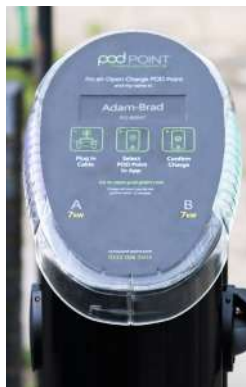
The display on a Pod Point charger. Usage statistics are communicated to a central hub
